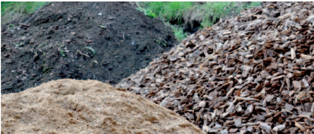
Backfill for planting: sand, topsoil and soil conditioner
