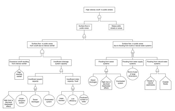
Figure 3 – Example of a fault tree for the hazard 'High velocity runoff in public streets'
