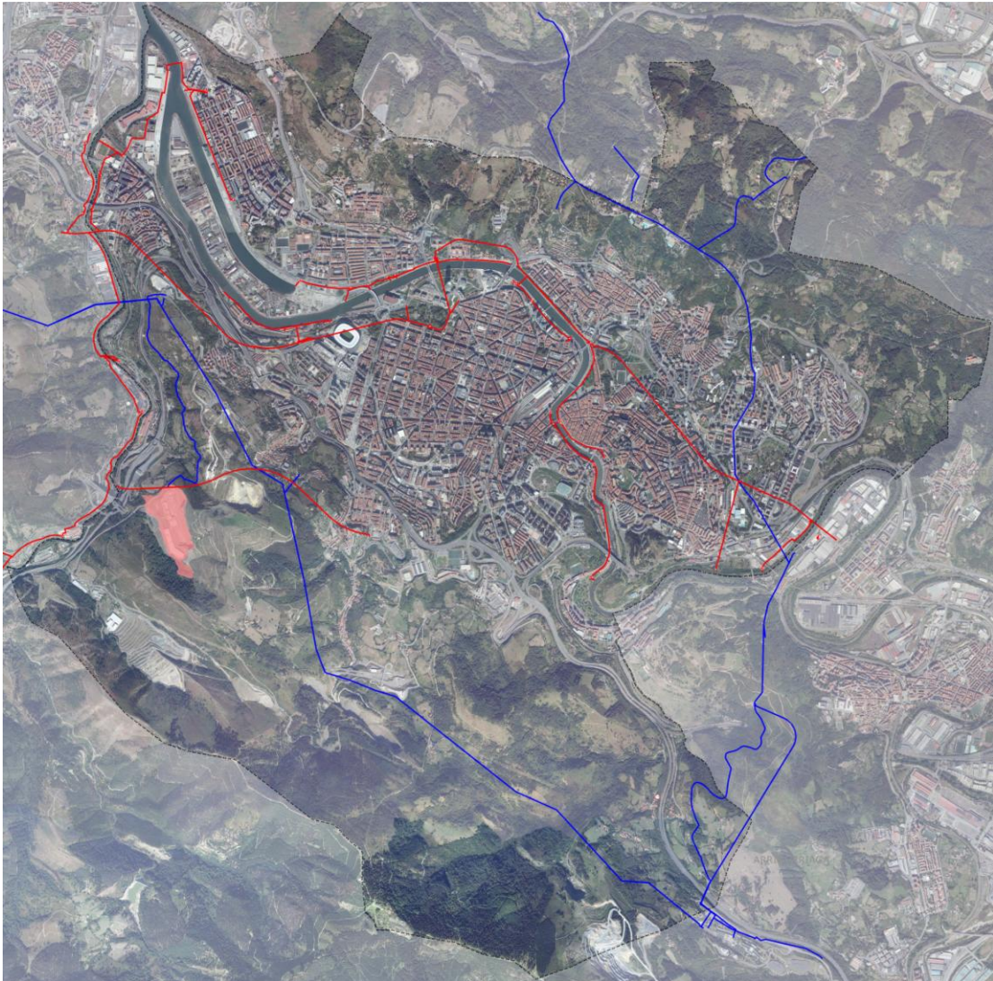
Fig. 4: Water supply and sewerage network (red lines represent the municipal network; blue lines the network of the Bilbao Bizkaia Water Consortium) and waste disposal site “Zabalgardi” (red area at left) (Town Planning Office, Municipality of Bilbao, 2015)
