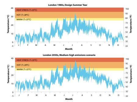
Figure 4: Daily temperature ranges in the CIBSE London Design Summer Year for the 1980s (upper panel) and 'morphed' ranges for the 2050s under the UKCIP02 Medium-High emissions scenario (lower panel).
