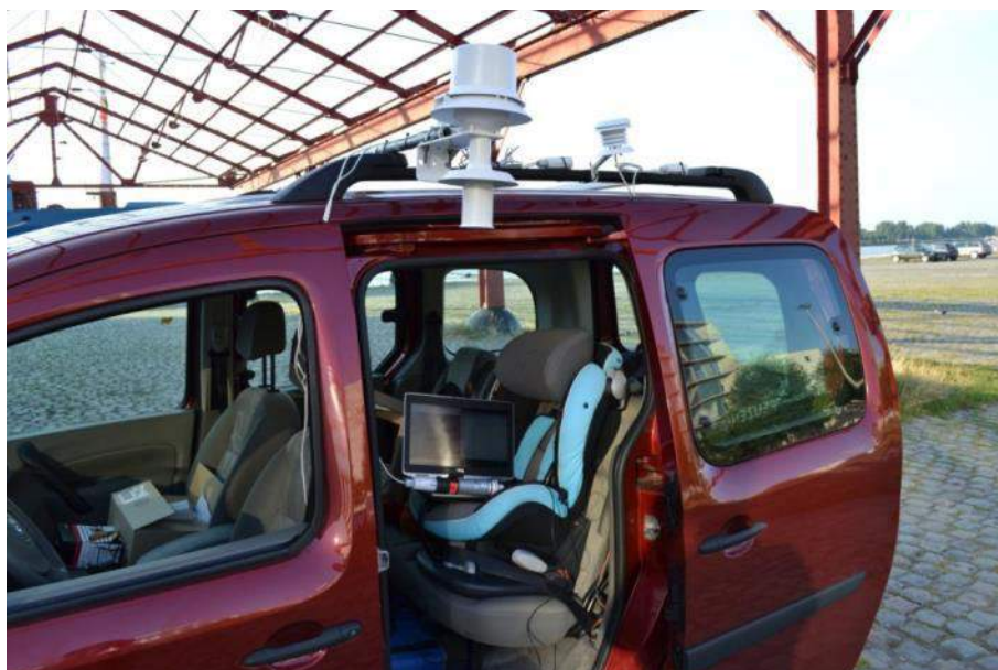
Figure 22 – Actively and passively ventilated temperature sensors, mounted on the car used as a mobile platform. The actively ventilated shield is powered by the car battery's 12 V connection. In the analysis below, we only use data from the actively ventilated measurements.
