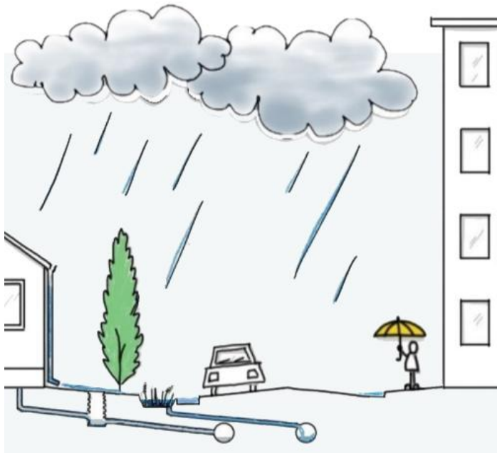
Figure 2: Handling rainwater in a separate system, using green roadside infiltration beds to delay rainwater, increasing drainage capacity and preventing overflows. In Risvangen the stormwater flows slowly into a nearby stream. Image Credit: Ane Mølgaard Rasmussen, Aarhus Vand (local water utility company).
