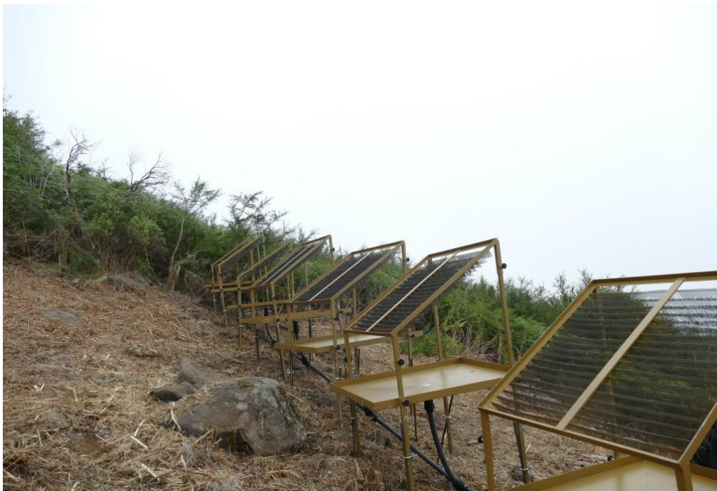
Figure 2: Fog water collectors with metal needles. Image Credit: Cabildo de Gran Canaria/David Delfour.
