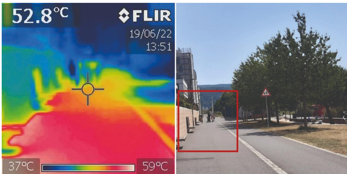
Figure 1: Infrared image of the surface radiation temperature on a hot day in July 2022 on the 'Promenade' in Heidelberg's 'Bahnhof' district. Image Credit: Foshag et al. (2024) .
