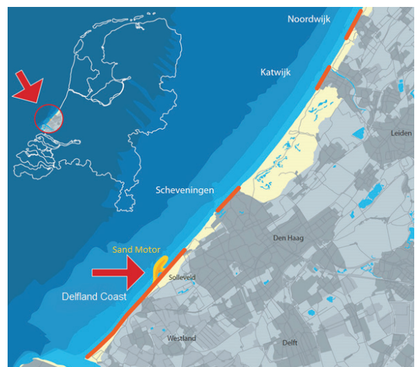
Figure 5. Location of the Sand Motor on the South Holland coast. In red, the Weak Links: the 'Delfland Coast' was reinforced in 2008-2009. Source: Vertegaal et al., 2016.
