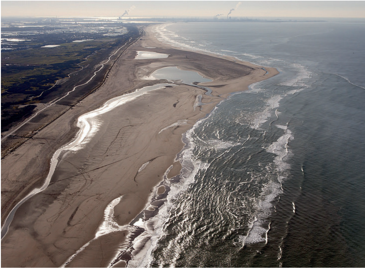
The Sand Motor on 16 February 2016, with the breach – one month old at the time – near the lagoon.
