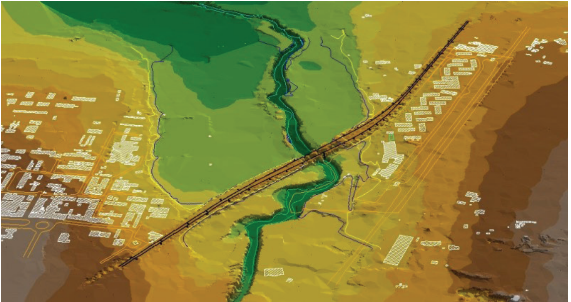
Image 2. A Computer generated image of a river, the 50- and 100-year flood lines (blue and yellow lines), a double line railway bridge and the existing surface infrastructure in the vicinity of the river © African Environmental Development
