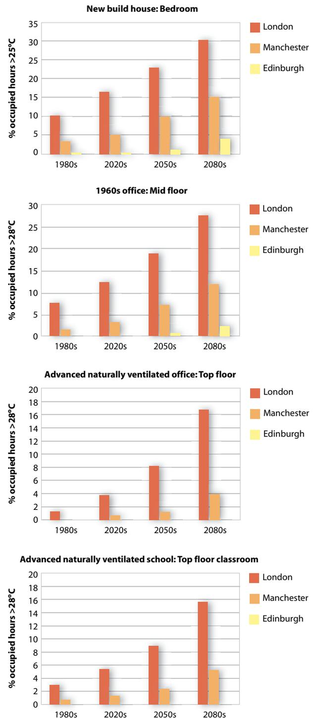
Figure 13: The percentage of hours that the 'hot' discomfort temperature is exceeded in four of the case study buildings.
